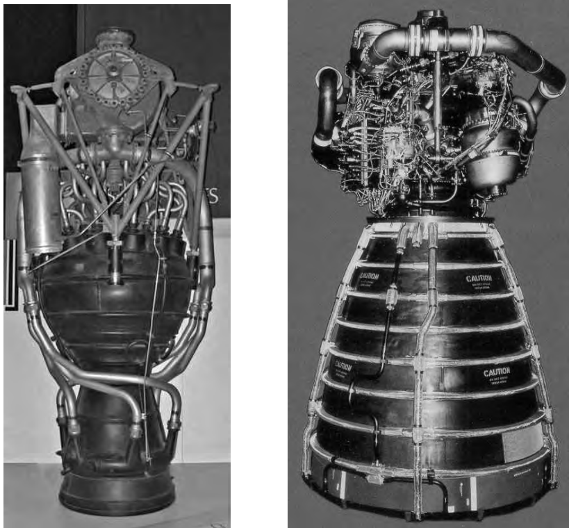
Figure 17.3. Left: A4/V2 rocket engine (circa 1943). Developed and used by Germany during the Second World War. After the war it was used to “ignite” the American rocket program. Engine height: 1.7 meter. Propellant: 75% ethanol and liquid oxygen. The V2 rocket was powered by one such engine. Image courtesy Wikimedia Commons. Right: Space Shuttle Main Engine (SSME); developed in USA (circa 1980). Engine height 4.3 meter. Propellant: liquid hydrogen and oxygen. The Space Shuttle was powered by three such engines, aided by two solid fuel boosters during lift-off. Image courtesy RocketDyne Archives (permission to be obtained).
