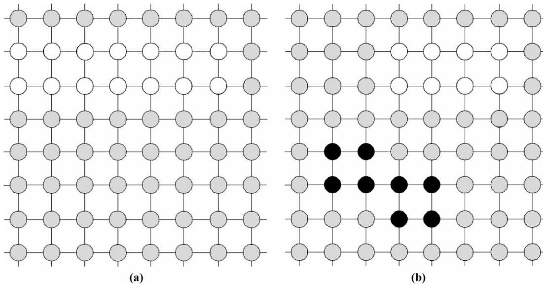
Fig. 2. Clusters of control sites for a 2D lattice. For a lattice with accidental degeneracy (a) the size of the minimal control cluster (white) grows linearly with the size of the lattice. If there is no accidental degeneracy, (b) the lattice can be controlled using a local cluster of control sites. Two examples of allowed minimal local clusters (white and black) are shown.
